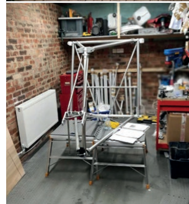
Right A Skyranger under construction. This aircraft is one of Britain's most popular kits (photos: Pete and Mandy Jenkins)
